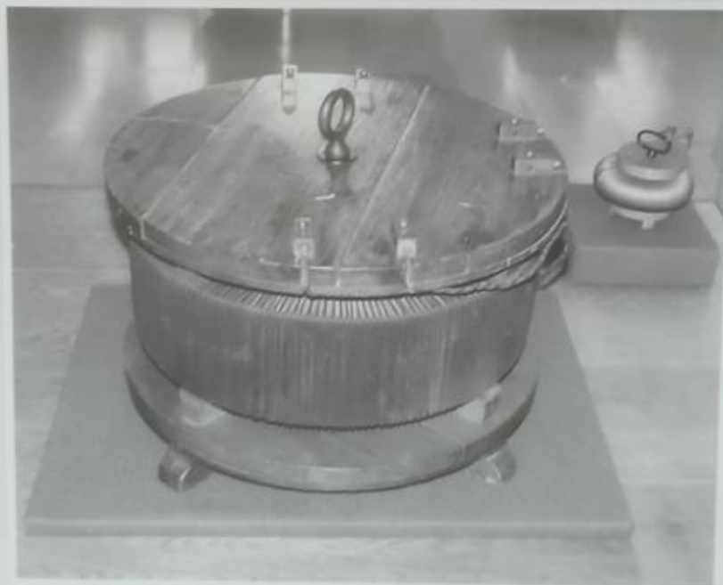
Prototypes of the world's first high-efficiency transformers, 1885
